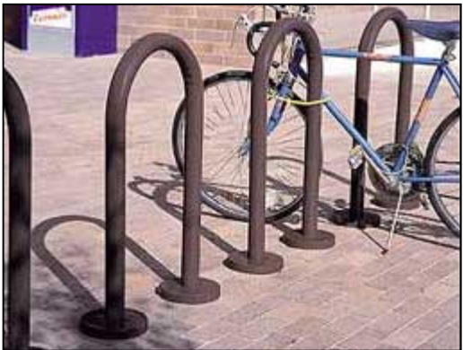
Bike Racks- Simple individual loop racks are more flexible for areas with minimal sidewalk space. The simple design is compatible with the other street furniture and should be painted to match other furniture.
