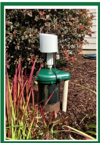
The monitoring system uses next-generation acoustic sensor technology to measure water levels in residential, agricultural, industrial and irrigation wells. This network involves adding compact water-level sensors to wells to measure the groundwater fluctuations in that area remotely. The sensor attaches to the top of the wellcap and won't interfere with the function of the well.
